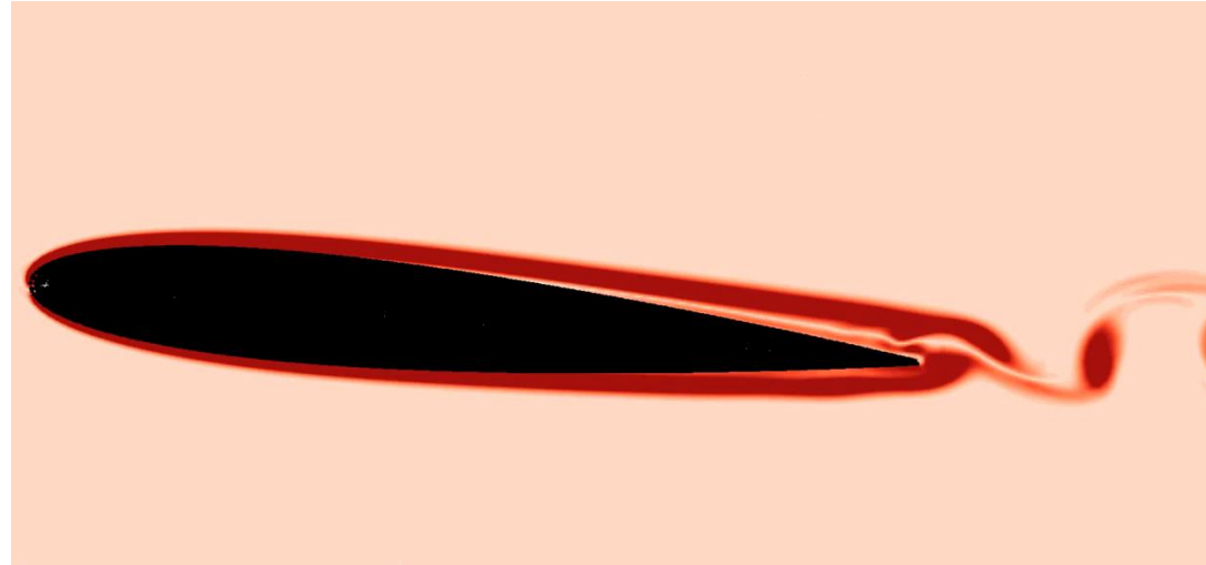
Pitching Airfoil under Dynamic Stall [Ouro et al., Journal of Fluids Engineering, 2018]
